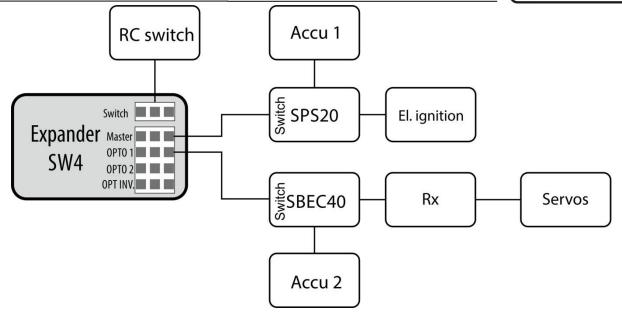
Fig. 1: Expander SW4 application connection
