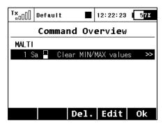
Using the menu item "Clear MIN/MAX values", you can assign any control or switch that will be used to clear minimums and maximums in the sensor.
