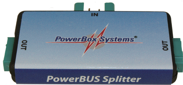
A PowerBUS splitter is employed if additional bus cables are required. As you can see there is one input and two outputs.
