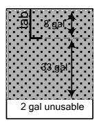
**Example B:** Aircraft has two MAIN and two AUX tanks.
