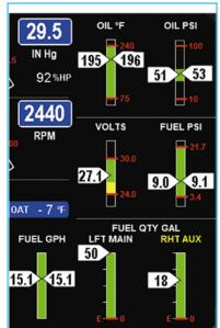
The range of the bar graphs depends on the programming. Range, redlines and/or limits are typically set to match the original aircrafts gauge markings. These are locked for Primary installations, however non-primary gauges can be user modified, using 'EDM Config' utility downloadable from <a href="www.jpitech.com">www.jpitech.com</a>. See 'Section 9 - First Time Setup and Customization'.
