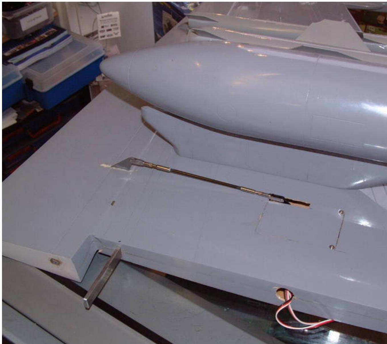
If you do not want to use the new Flaps system, you will need to cut the holes for install the Flaps servos
