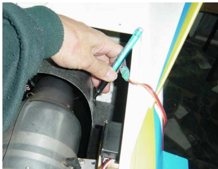
**make the by-pass holes to fasten the dual wall tail pipe**
