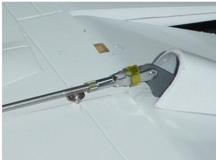
**connect both push-pull rods for Aileron servos control (the F-18 kit includes 2 rods for Ailerons)**
