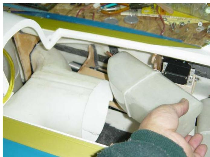
**first: Take out the cross spar for install both Fuel Tanks**
