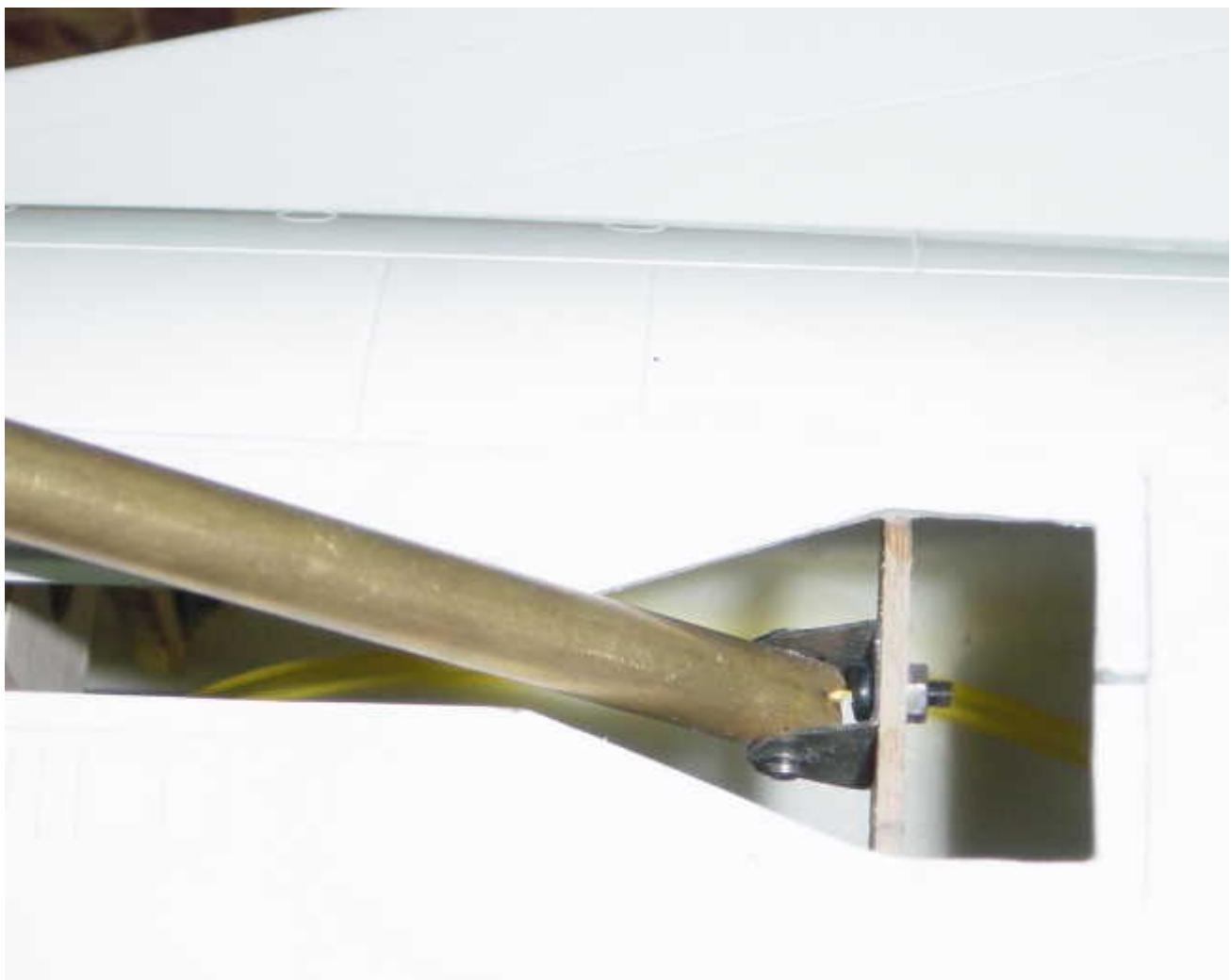
**install nose gear with after connecter**
