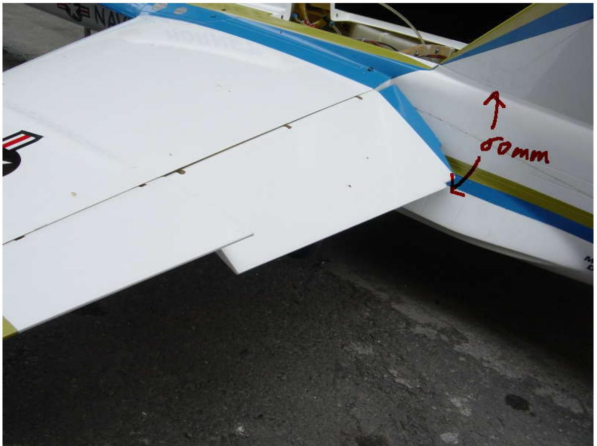
**set-up Flaps function for down movement 60mm for Landing**
