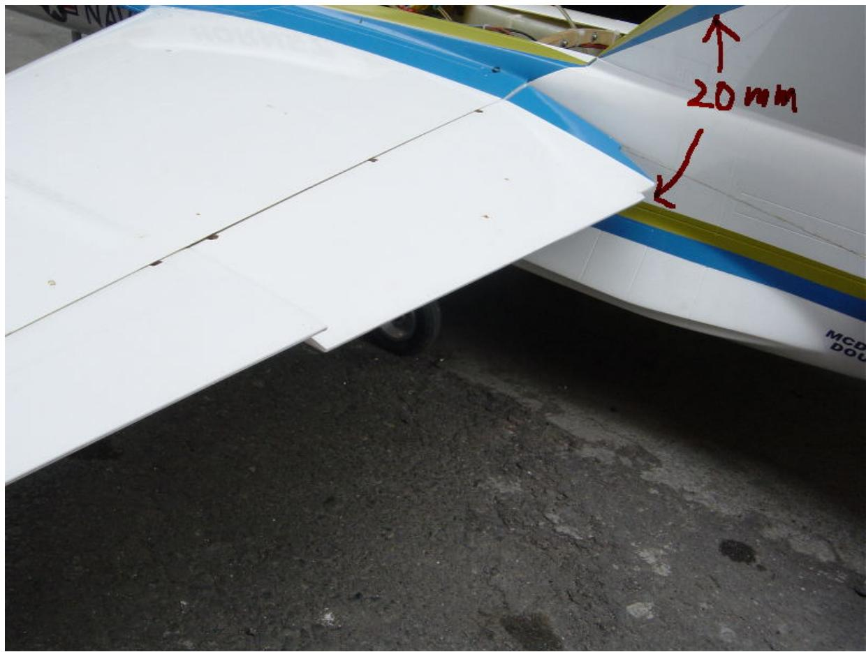
**set-up Flaps function for down movement 20mm~ 25mm for Take off**
