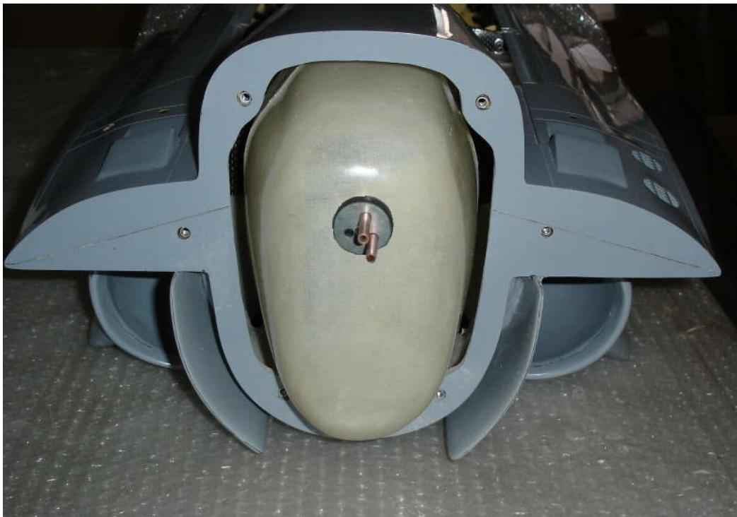
**install front fuel tank before installing nose cone**
