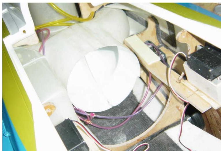
**install main gear with setup air pipes for air breaks for the main gear**
