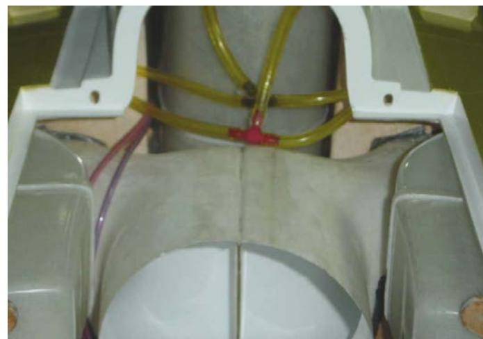
**setup fuel pipe with "T" fitting for connect to both fuel tanks with over follow**
