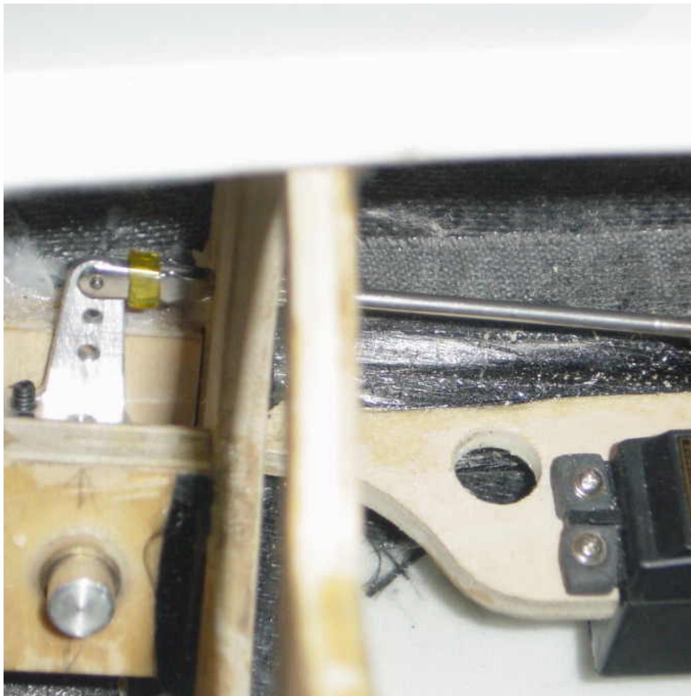
**connect both push-pull rods for elevator servos control (the F-18 kit includes 2 rods for Elevators)**
