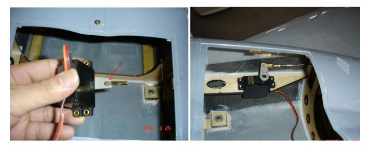
connect both push-pull rods for elevator servos control
