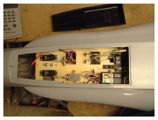
install the retracts control servo with break control servo, install two (2) valves for jet engine with the fuel pump
