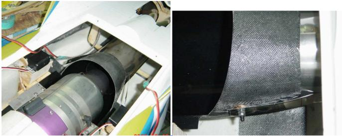
make the by-pass holes to fasten the dual wall tail pipe
