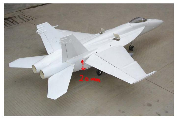
set-up Flaps function for down movement 20mm~ 25mm for Talk off
