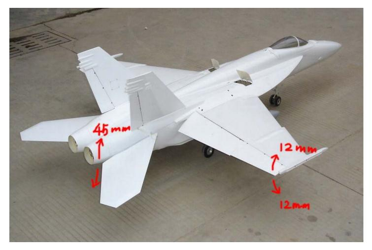
set-up ailerons function for up / down movement for each to between 12 mm ~ 16 mm set-up elevator function for up / down movement for each to between 40 mm ~ 45 mm
