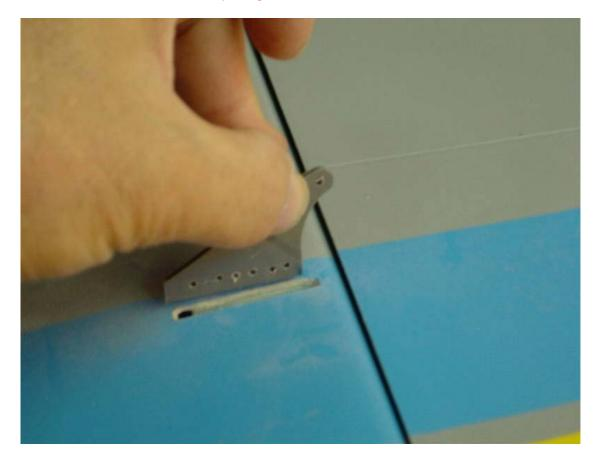
Glue the servos mounts for the Aileron servos and cut the hole then glue for Rudder Horns connect both push-pull rods for Aileron servos control (the F-18 kit includes 2 rods for Ailerons)
