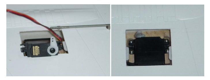
install the aileron servos, We suggest use of the JR # 3421servos for the ailerons
