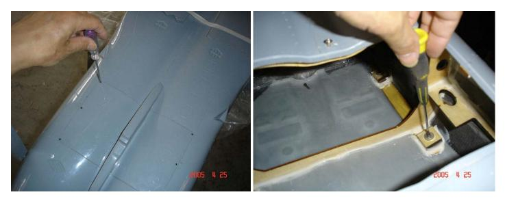
Take out the 6 screws and Bottom Cover and install the Rudder Fin
