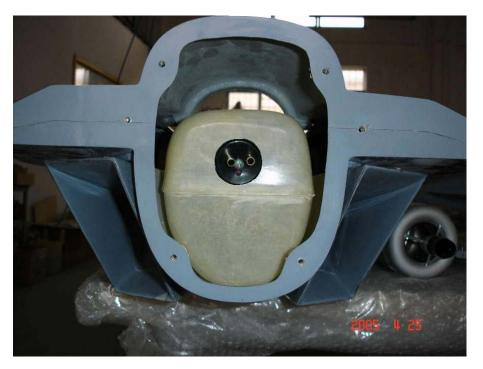
install front fuel tank before installing nose cone
