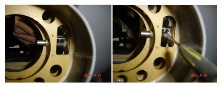
elevator shafts and servo arms must be installed first (make sure that there is a minimal lateral movement) and after which the servos mounts can be installed (included in the kit).
