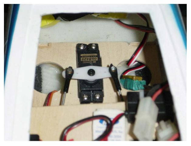
setup the front servo and make two piano wires control to the nose gear
