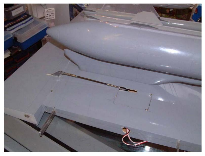
If you do not want to use the new Flaps system, you will need to cut the holes for install the Flaps servos
