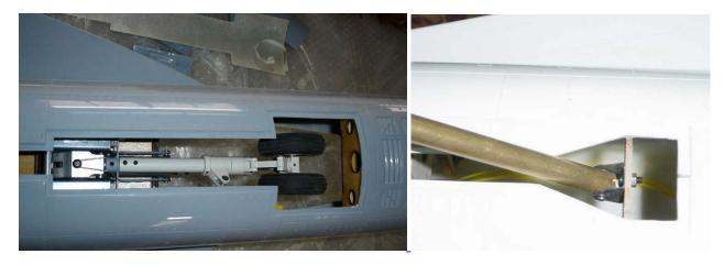
install nose gear with after connecter
