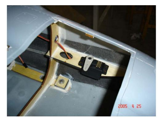
install two servos for the Elevators
