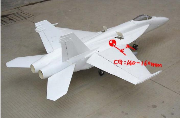
set-up elevator function for up / down movement for each to between 40 mm ~ 45 mm
