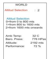
To set the local altitude enter the value corresponding to your local altitude, the values are 0 through 2, the ECU measured altitude which is displayed on the lower section of the display should be used as a reference.
