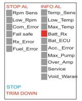
"Temp\_Sens" indicates a temperature probe failure
