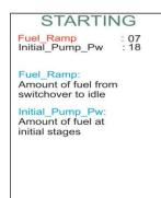
There are only two adjustable parameters in this sub-menu, "Initial pump Pw" values and "Fuel Ramp".
