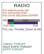
To program the throttle stick position value into the ECU select "Ok" on the HDT. Move your transmitter trim up all the way and your throttle stick down; then press "OK" on the HDT.
