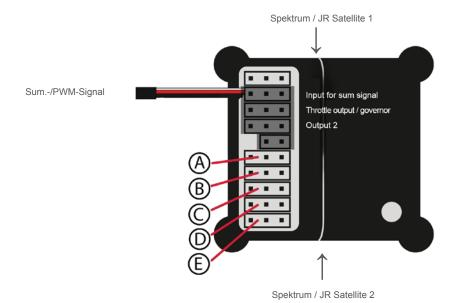
To use a serial connection (sum signal) the input mode of the system must be configured as per PC setup software. The channels on the PC are assigned in the same way. The setup software is also suitable for binding Spektrum/JR satellites. Furthermore, the setup software offers a very easy-to-understand test option for all received signals with its Diagnose page.
